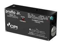
The Proflo® Jr. monitoring device provides shutdown protection for your compressor based on the operation of the cycle times of the divider block system.
