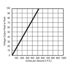
Note: Tested at 1000 I.P.S. 20 pitch gear, 0.005 gap and 100K OHM load.
